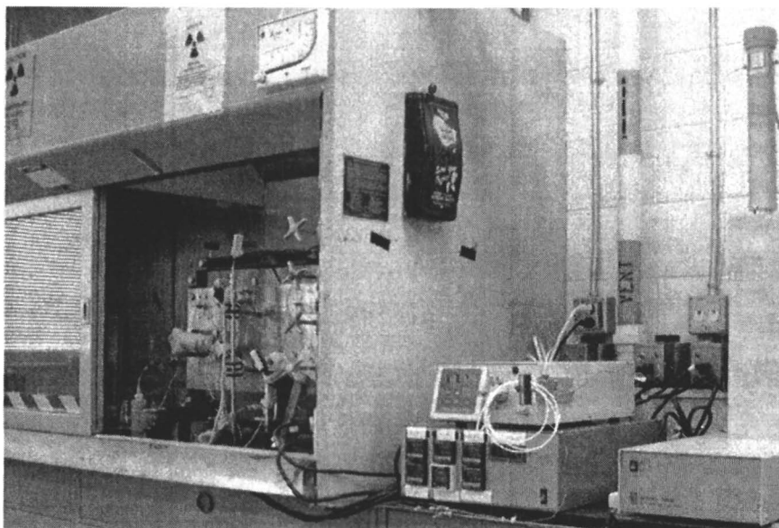
Figure 2. Photograph of the SFE System in a radiological control hood.
